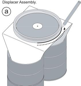
Remove the Cylinder Ring, place it on a piece of heavy paper or cardboard and trace it's inner and outer outline onto the paper.
