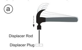
Press the Displacer Rod and Displacer Plug into the hole in the Yellow Displacer Foam
