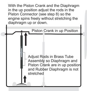
Observe the motion of the rods on the Crankshaft as you slowly rotate the Propeller. Is it binding? If so, figure out where the binding is and adjust the connectors accordingly. Binding is usually caused by the Displacer hitting the Crankcase or the Cylinder Cap, or by the Piston being stretched. When you have everything working smoothly, spin the Propeller quickly by hand. The Propeller should spin about four or five revolutions before stopping
