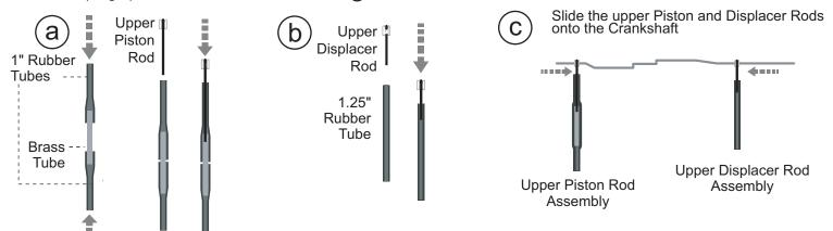
The small gray plastic bearings installed in the Crankcase must be free from flash and other defects. If necessary, ream them out by hand with either a 1/16 inch, #52, or a 1.5 mm drill bit. Install the Crankshaft in the Crankcase so that the Upper Displacer Rod is over the center of the engine and the Piston Rod is above the Piston. Later, when you are ready to run the engine, you will be tempted to oil these bearings. Do NOT do this. The engine runs much better with no oil on the bearings.
