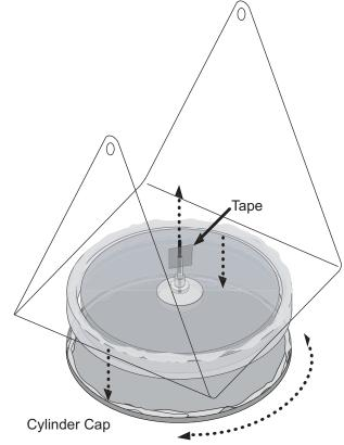
Carefully apply a bead of Silicone Sealant or Epoxy just inside the lip of the Cylinder Cap. Gently press and twist the cylinder into the Cylinder Cap to seat it in the glue and eliminate gaps. Let it dry.
