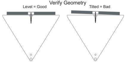
If you are using caulk or epoxy, apply a small amount of adhesive to the edge of the plug and press it into the inside of the Displacer (yellow foam disk). If you are using super glue, assemble the parts dry and then put three drops of Superglue equally spaced around the Plug; then wipe any excess glue off. After verifying the geometry of this assembly set the Displacer assembly aside to set/dry. The next step is to install the Displacer and glue the Cylinder Cap.
