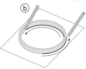
Using the lines traced from the Cylinder, generously apply Silicone Sealant or carefully mixed Epoxy between the traced lines.
