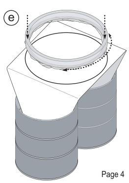
After the joint between the Crankcase and the Cylinder Ring has dried, secure the Displacer assembly in the up position with a piece of tape or the rubber tubing (to keep it from being glued to the Cylinder Cap).
